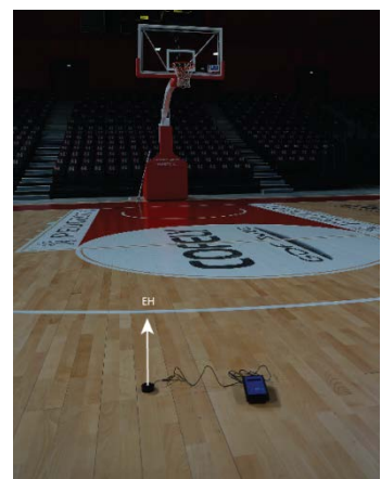
Horizontal illuminance (EH) measurement
