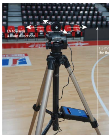
Vertical illuminance (EV) measurement
