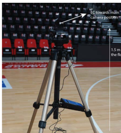
Main camera illuminance (EC) measurement
